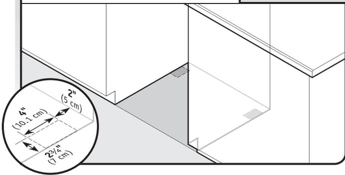
Built-up floors (Kitchen floor height is higher than cabinet opening.) Example: Kitchen floor tile does not extend into cabinet opening. Add shims as needed in the area shown to bring the dishwasher up to 34" (86.4 cm) below the countertop.
